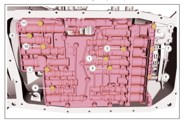
Main control bolts should be tightened to 8 Nm (71 lb-in) in the sequence shown
